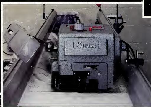
Knotex Warp Tying Machine —Speeds to 600 knots per minute. Ties knots with tails from 1/4" to 2 1/4". Tying methods include lease-to-lease, lease-to-flat and flat-to-flat. Ties all fibers.
